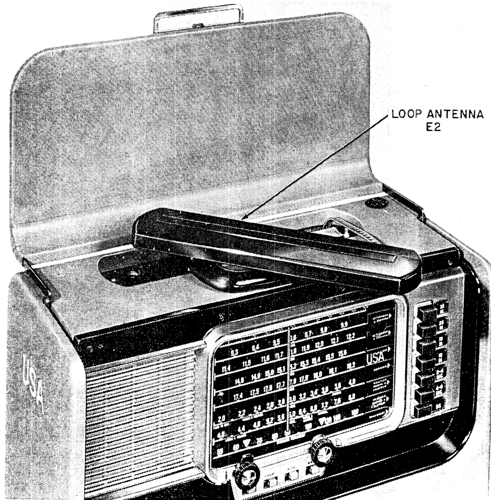
Figure 9.2. Location of loop antenna for orientation for Radio Receiver R-520A/URR.
